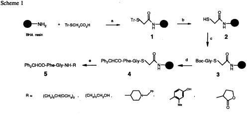
Reagents and conditions: (a)BHA resin (0.86 mmole/gr), Ts-CH<sub>2</sub>COOH (4 eq.), DCC (2 eq.), DMF/DCM(1:2 v/v), 24 hrs; (b) TFA/DCM/Et<sub>3</sub>SiH (5:5:1, v/v); (c) Boc-Gly-OH (4 eq.), DCC/DMAP (1:1, 4 eq.), DCM, 24 hrs; (d) TFA/DCM (1:1) then Ph<sub>2</sub>CHCO-Phe-OH (4 eq.), HBTU/HOBT (1:1, 4 eq.), DIEA (12 eq.); (e) R-NH<sub>2</sub> (3 eq.), i-propanol, 75°C, 24 hrs.
